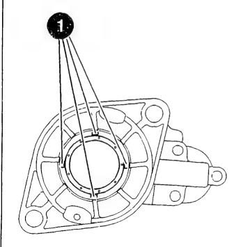
COMPONENT CHECKING AND REPAIR Checking drive-end shield (version with needle bearing) Radial lip-type oil seal and bushing of drive-end shield are always to be replaced. Removing radial lip-type oil seal: Clamp drive-end shield (1) in clamping support. Use suitable tool to prise out radial lip-type oil seal (2).
